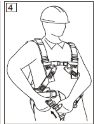
4 Pull one and then other thigh straps through crotch, take care do not twist them.
